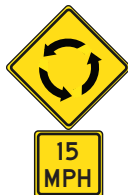
Speed Advisory At Roundabout
